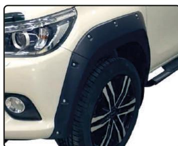
EXTENSIONS D'AILES AVEC RIVETS
